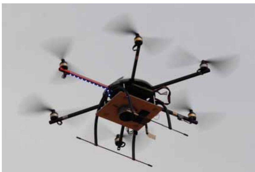
Figure 1: The hexacopter used in data collection. The camera is mounted under the vehicle.
