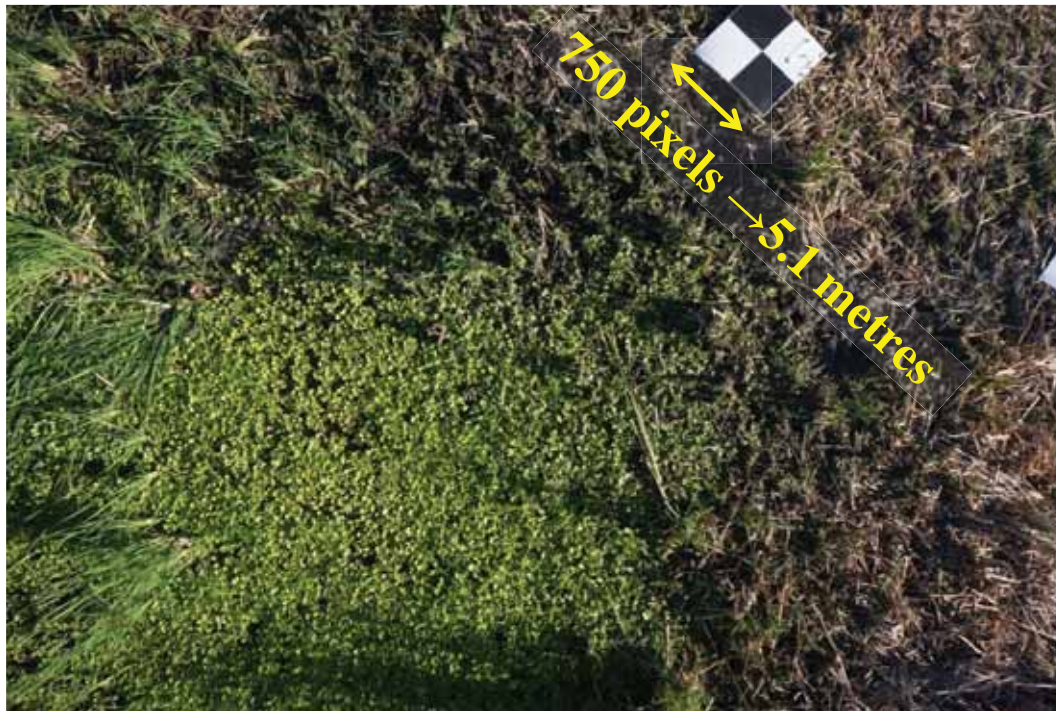
Figure 2: Estimating the flight altitude using a checker board
